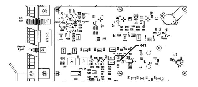
Unsolder A4R41 and replace it with the 162 ohm resistor. Use extreme caution since this is a surface mount component. Although probably not necessary, it is generally a good idea to redo adjustments #104 through #109. If the problem existed even when the analyzer was not in dither mode, then performing these adjustments is definitely required.
